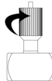
Turn knob counter clockwise (to the left) to open
