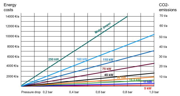
Assumptions: 8000 Bh/a, 0,1 €/kWh, Power loss per bar 8%, Power plant emissions 0.545 kg CO2/kWh
