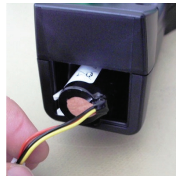
Carefully pull out the battery
