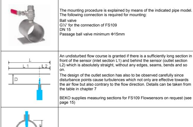
The sensor has to be inserted centrally into a straight piece of pipe.
