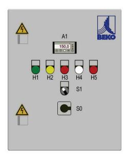
Α1 Temperature controller S0 Main switch S1 Starting switch Converter operation / "Green" light H1 H2 ALARM: Temperature monitor AUTO-RESET / "Yellow" light ALARM: Safety temperature monitor Н3 AUTO-RESET / "RED" light H4 Reactor heating phase BEKOKAT® AUTO-RESET / "White" light
